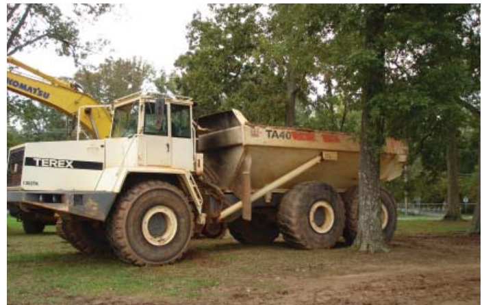
Figure 9. Construction equipment contributing to tree decline by soil compaction.
